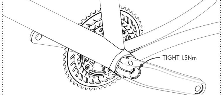
Grease and install the crankset following the manufacturer's assembly steps.
