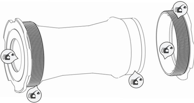
Apply grease to the indicated contact surfaces.
