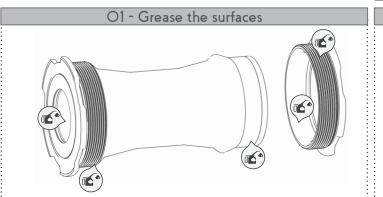
Apply grease to the indicated contact surfaces. Including the surfaces in contact with the connecting rod.
