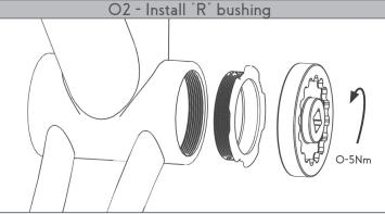
Install the right side. With the help of the 'assembly wrench' apply up to 5Nm. DO NOT OVERTIGHT.
