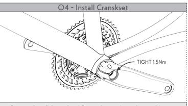
Grease and install the crankset following the manufacturer's assembly steps.
